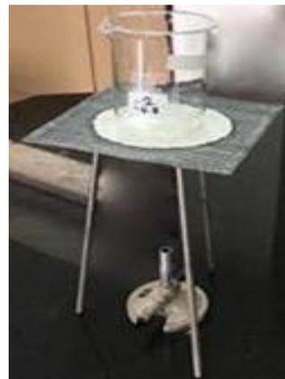
Figure 2: Gauze mat sitting on tripod over Bunsen burner.
